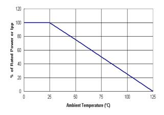
Figure 2. Power Derating Curve
