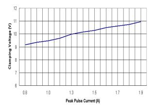
Figure 1. Clamping Voltage vs. Peak Pulse Current
