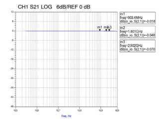
Figure 4. Insertion Loss S21 - I/O to I/O
