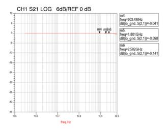
Figure 3. Insertion Loss S21 - I/O to GND
