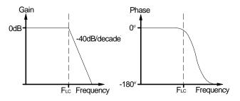
Figure 5 - Gain and phase of LC filter.
