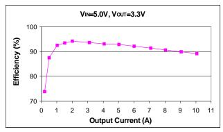
Figure 21 - Efficiency for IRU3037 Evaluation Board.
