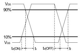
Figure 4 - Switching time waveforms.
