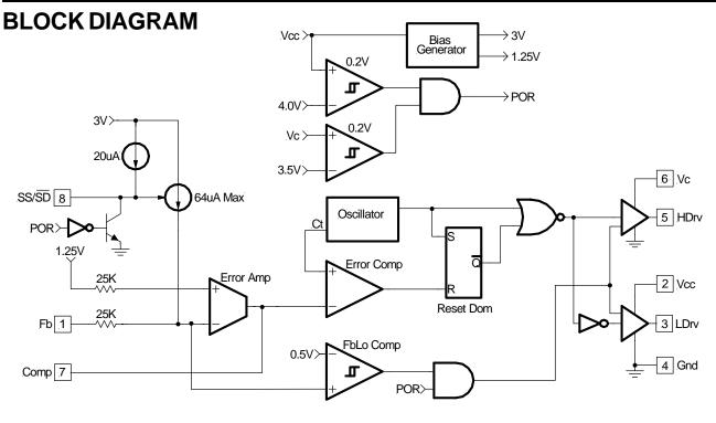
Figure 2 - Simplified block diagram of the IRU3037.
