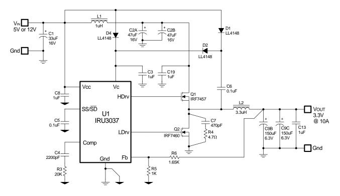
Figure 20 - Demo-board application of IRU3037.
