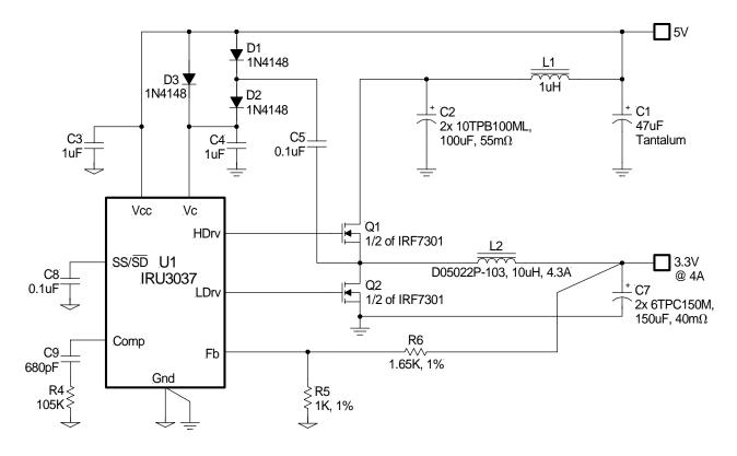
Figure 17 - Typical application of IRU3037 in an on-board DC-DC converter using a single 5V supply.
