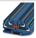
Disconnect terminal block, with isolating plug, Connection type: Push-in connection, Cross section: 0.14 mm² - 4 mm², AWG: 26 - 12, Nominal current: 16 A, Nominal voltage: 400 V, Length: 92.4 mm, Width: 5.2 mm, Color: blue, Assembly: NS 35/7,5, NS 35/15
